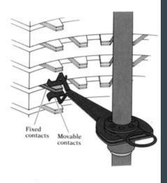
The movable contacts in a step-by-step switch can connect to any of a 100 different pairs of fixed contacts, each leading to a different line.
